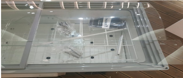
fig 7. Hyperstructure (type 2), hyperstructure adjusters (set 2), handles, lighting (tube), handles
