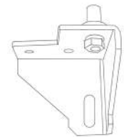
9. Remove the bottom hinge pin and turn the bottom hinge 90 degrees.
