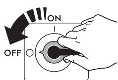
Disconnect the appliance from the power supply before carrying out any installation, assembly, cleaning or maintenance procedure.
