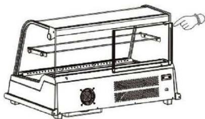
8. Install the internal sliding glass doors in the rear part of the device.
